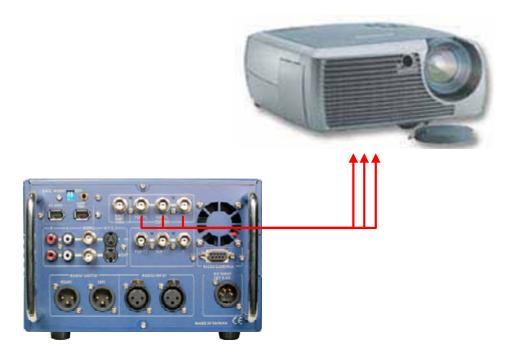
3. Connecting Y/C or Composite video and stereo audio outputs from an analogue camcorder or DVD player to the MP-6000.
